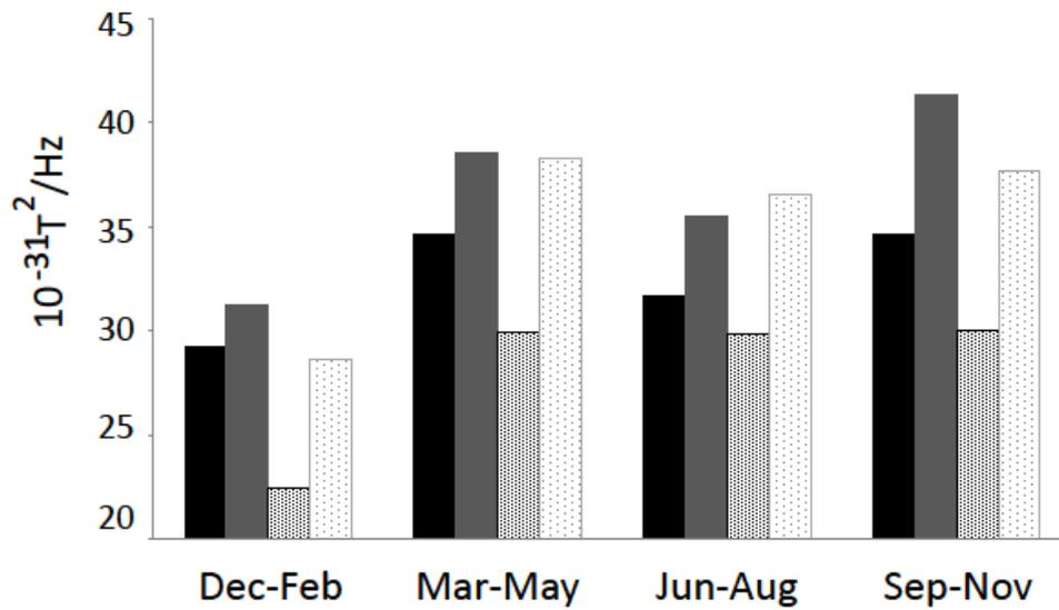
Figure 1. Ground VLF power following storms averaged by season. Black bars: VLF averaged over 0-48 hours following minimum Dst. Gray bars: VLF averaged over late recovery (48-72 hours following minimum Dst). Solid bars: VLF averaged over all hours of the day. Patterned: VLF averaged over the dawn period (9-12 UT).
