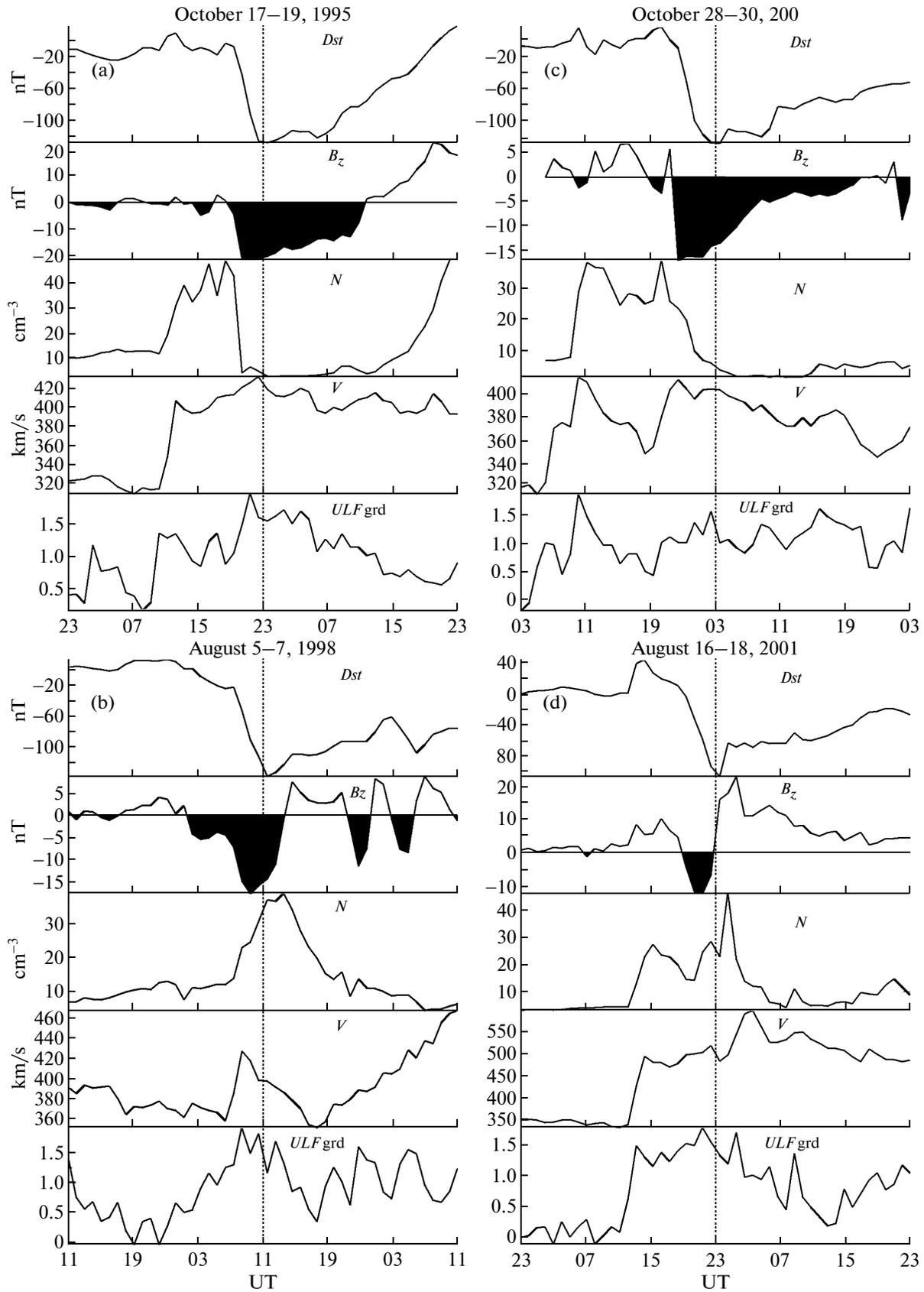
**Fig. 3.** Examples of variations in the  $Dst$  index IMF  $B_z$  component, solar wind density ( $N$ ) and velocity ( $V$ ), and the ground-based  $ULF$  index during four magnetic storms.
